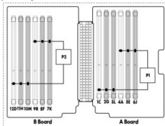
The memory subsystem in this server is divided into channels. Each processor supports eight channels, and each channel supports three DIMM slots, as shown in the table below. White DIMM slots denote the first slot of a channel (Ch 4A, Ch 9B, Ch 1C, Ch 12D...).
